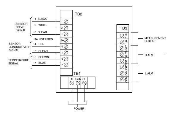
Figure 8. Rear Panel Wiring - Plastic Enclosure
