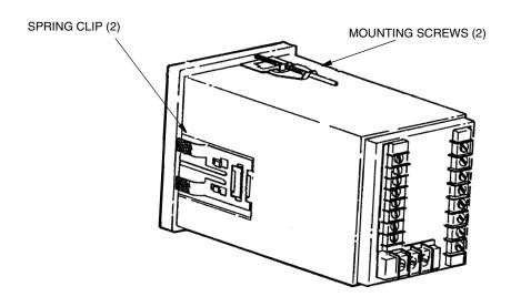
Figure 3. Mounting to Panel - Plastic Enclosure
