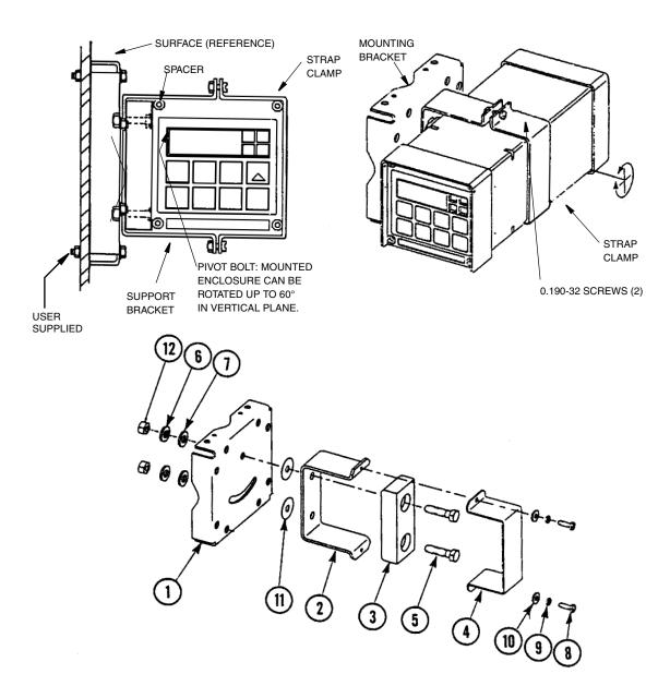
Figure 6. Metal Enclosure - Fixed Mount
