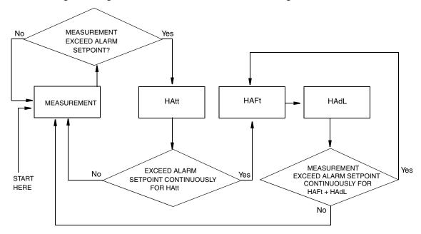
Figure 13. Flow Diagram for Alarm Timer Logic
