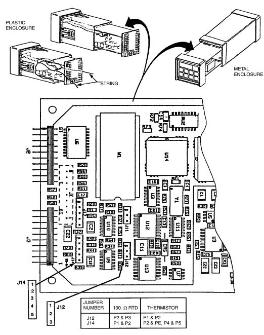
Figure 16. Jumpers for Temperature Compensation
