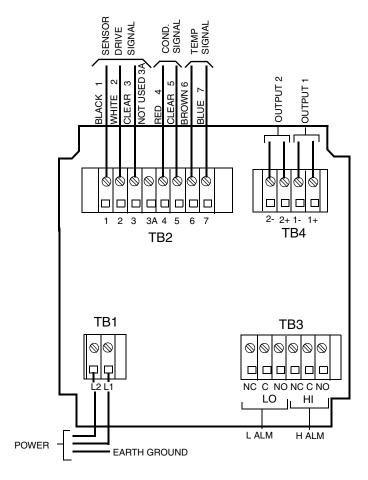
Figure 9. Rear Panel Wiring - Metal Enclosure
