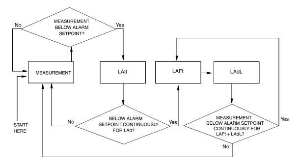
Figure 15. Flow Diagram for Alarm Timer Logic
