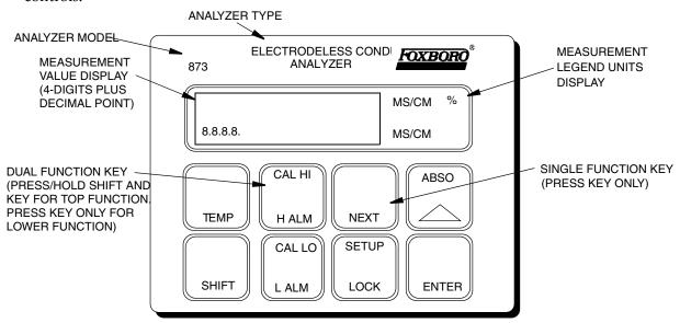
Figure 1. Front Panel Display and Keypad
