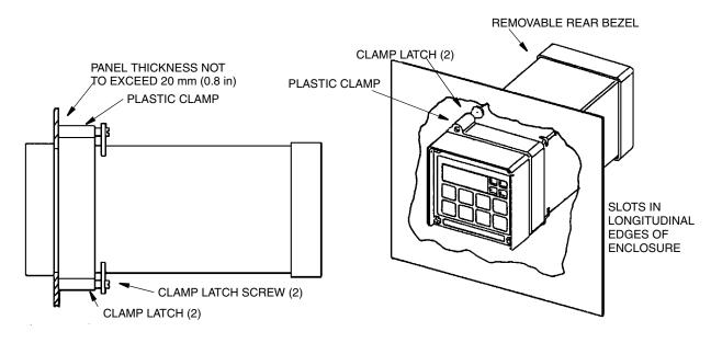
Figure 4. Mounting to Panel - Metal Enclosure
