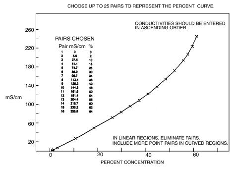
Figure 26. Concentration vs. Conductivity Data
