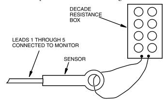
Figure 27. Sensor/Decade Box Configuration for Calibration
