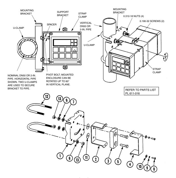
Figure 5. Metal Enclosure - Pipe Mounting
