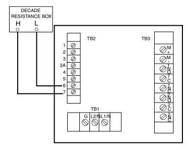
Figure 18. RTD Temperature Simulation (Plastic Enclosure Shown)
