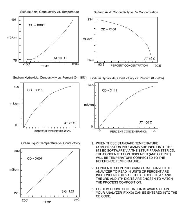
Figure 11. Sample 873EC Temperature and Concentration Curves
