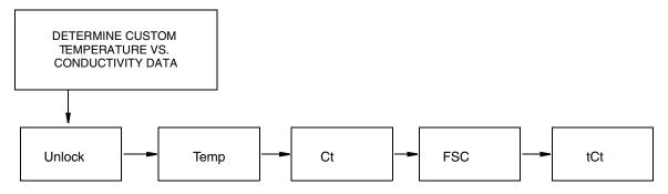
Figure 21. Flow Chart for Custom Temperature Compensation Curve (tCt)
