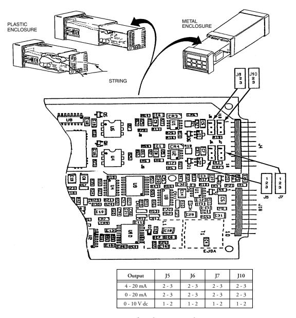
Figure 19. Jumpers for Changing Analog Output
