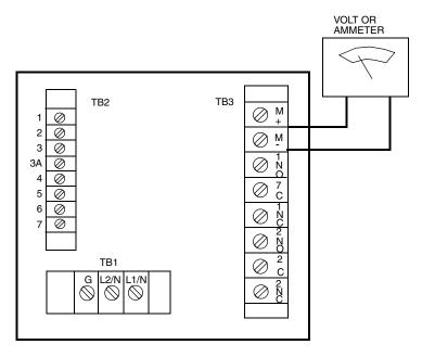
Figure 20. Output Terminals and Volt/Amp Meter (Plastic Enclosure Shown)
