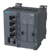
SCALANCE X308-2M; managed IE switch, compact; 4x 10/100/1000 Mbit/s for RJ45 ports electrical; 2x 100/1000 Mbit/s for 2-port media modules, electrical or optical; LED diagnostics; error signaling Contact; Select/set button; PROFINET IO device; network management; Integrated redundancy manager; office features (RSTP, VLAN, IGMP,...); C-plug in scope of delivery
