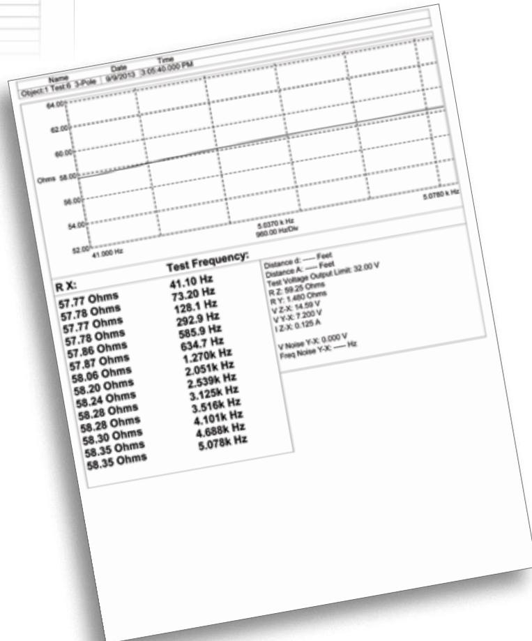
DataView® software provides a convenient way to configure and control ground resistance tests from your computer. Through the use of clear and easy-to-use tabbed dialog boxes, all ground tester functions can be configured and tests can be initiated. Results can be displayed in real-time and stored in your PC. Reports may be printed along with the operator's comments and analysis.
