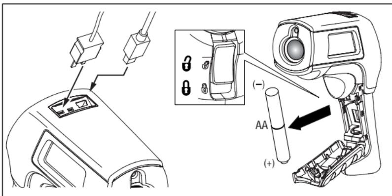
**Figure 2. Thermocouple and USB Connection and Changing Batteries**
