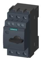
Circuit breaker 6.3 A A-release 4.5...6.3 A, N-release 82 A, for motor protection, class 10, screw connection, standard switching capacity w. transverse AUX. switch 1 NO + 1 NC
