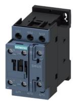
Contactor AC 230 V 50/60 HZ AC3 4 kW 400 V AUX contacts 1 NO +1 NC 3-pole, size S0 screw terminal
