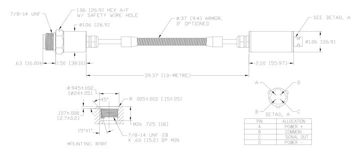
Figure 2: 165855-AA Cylinder Pressure Transducer and bore per SAE J1926
