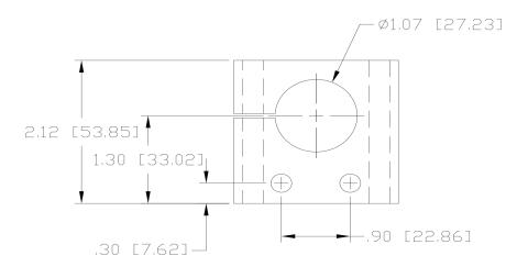
Figure 5: 29660-01 Mounting Clamp, use with M6 or 1/4-20 (not supplied)
